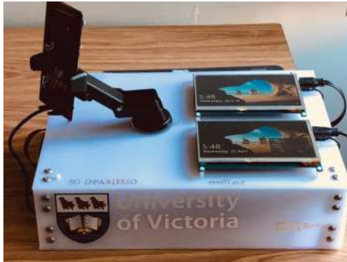
Fig. 5. 5G mmWave DPA-MIMO proof-of-concept system design.
